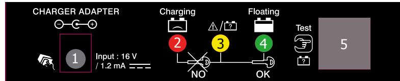
**1** Connection for the charger-adapter. Use only the charger-adapter provided with the product.
